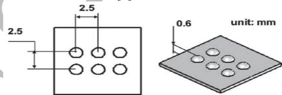
Fig. 2 - International building standard for a Braille cell
