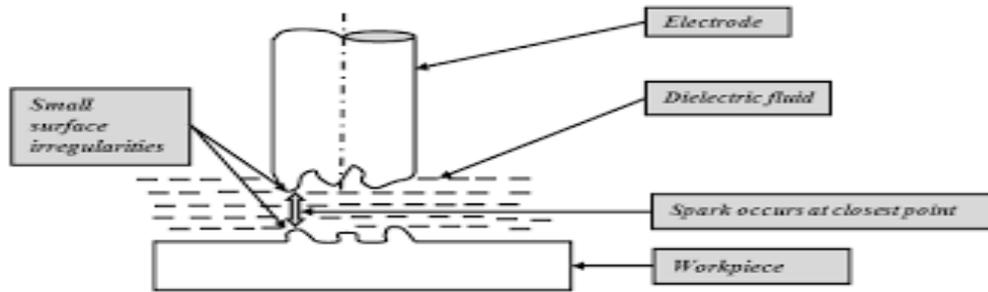
Fig: 1 Working Principle of EDM
