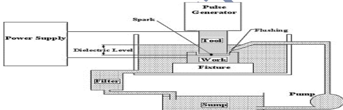
Fig 2: Schematic Setup of EDM
