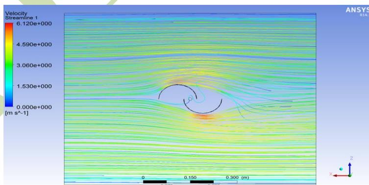
**Figure 4: Velocity streamline (left to right)**
