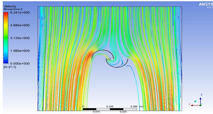
**Figure 2: Velocity streamline (top to bottom)**
