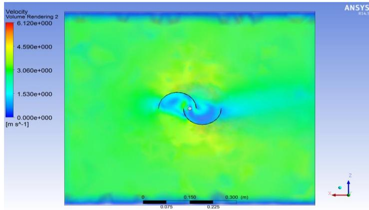
**Figure 5: Velocity volume rendering (left to right)**
