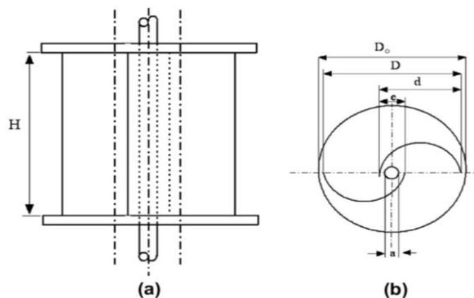
**Figure 1: 2D diagram single-stage Savonius rotor: (a) elevation view; (b) plan view**
