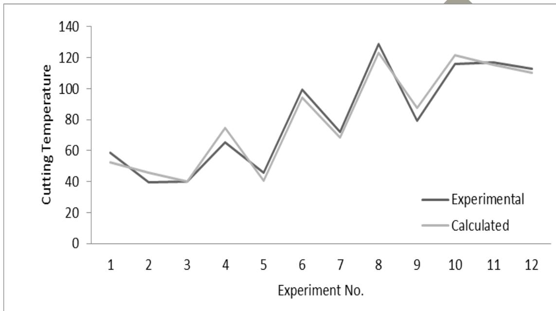
**Figure 2 Validation of cutting temperature model**
