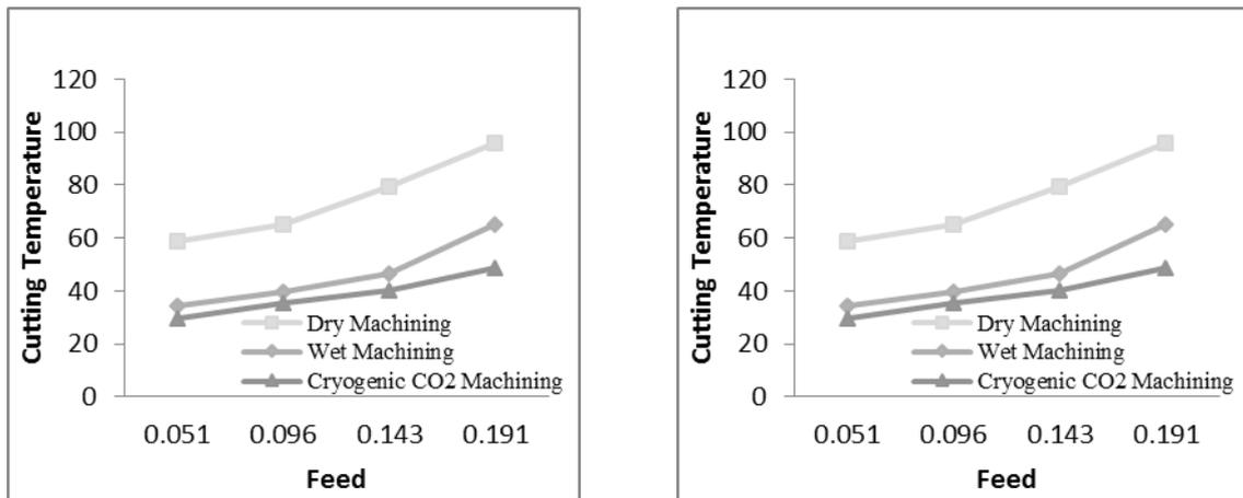
**Figure 3 Variation of the cutting temperature while machining AISI 1045 steel with different feed rates under different machining conditions (a) 41 m/min (b) 94 m/min**
