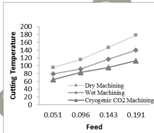
**Figure 3 Variation of the cutting temperature while machining AISI 1045 steel with feed rates 145 m/min under different machining conditions**
