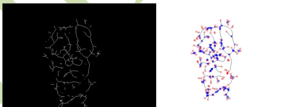
Fig. 7 a. Thinned image , Minutiae extracted image
