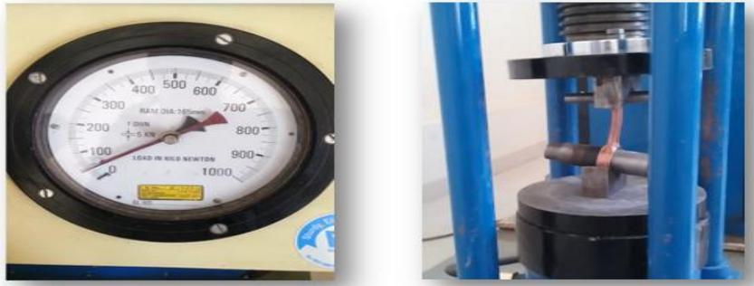
**Fig -4 Load on connecting rod during bending**
