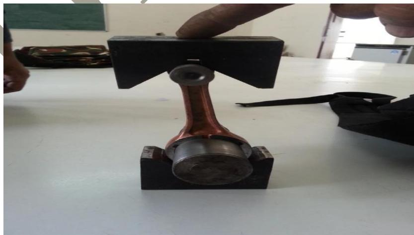
**Fig -3 Connecting rod with V-block**
