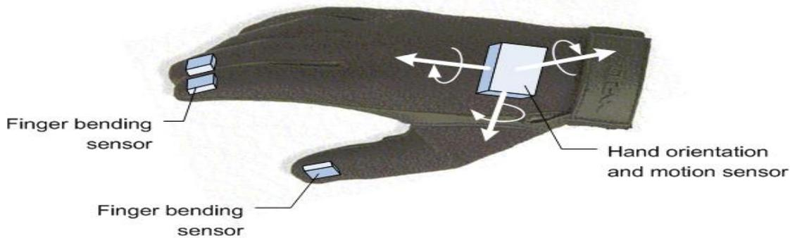
**Fig. 2. Data glove sensor layout**
