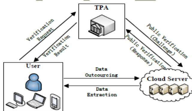
This system allot his schemed the client to initialize their privacy parameters and transmit the certification and Meta Cloud users information packets to TPA in the initial set-up phase and then the TPA verifies the validity of proof value generated by the server. Above all, this approach can protect the integrity and confidentiality of Cloud user's information packets in the Cloud computing server.
