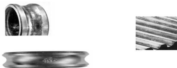
**Fig: Effects of contact stresses**
