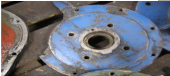
Figure 1.6 Breakage of Flange
