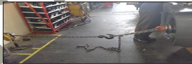
**Fig 1.5 Pull the Shaft through guide side**
