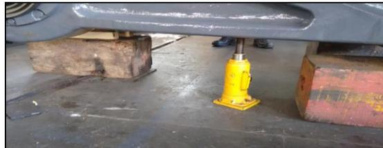
**Fig 1.3 Jack used to align the Jaw bore**
