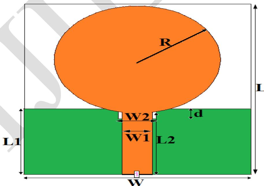
Figure 1. Geometry of antenna
