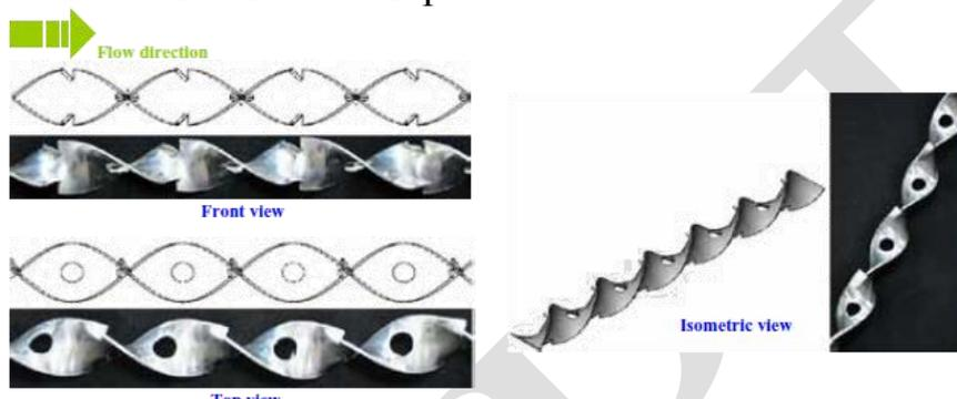
**Figure 4 Photograph and Sketch of Perforated Twisted Tape with parallel wings**
