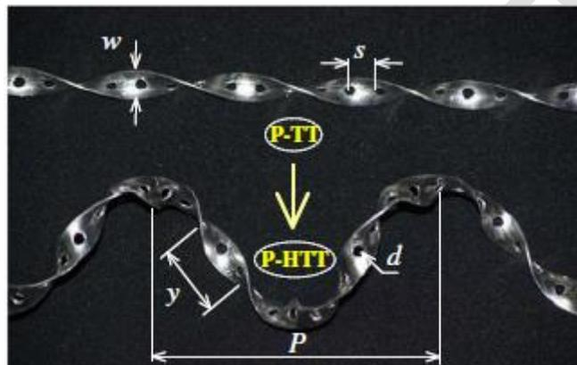
Figure 5 Perforated Twisted Helical Tape
