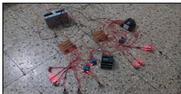
Interfacing of sensors and relays with PLC
