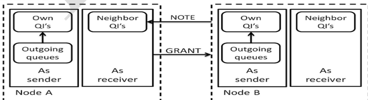
**Figure 1:- Block Diagram of Components in proposed modified MAC Protocol**
