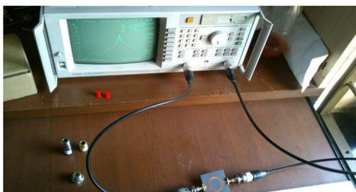
Figure 2: Permittivity Measurement Set Up
