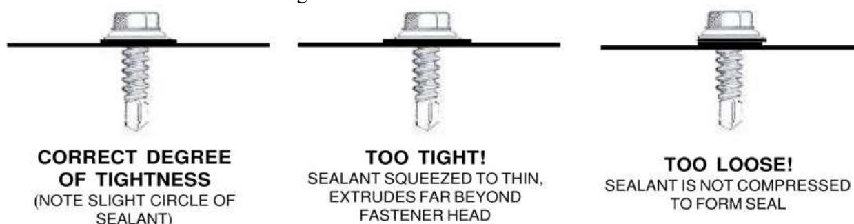
**Figure-10: Fasteners tighten system.**
