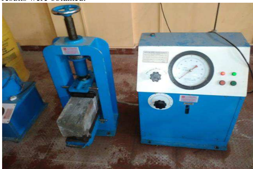
Fig 5.1 Beam loaded for flexural strength
