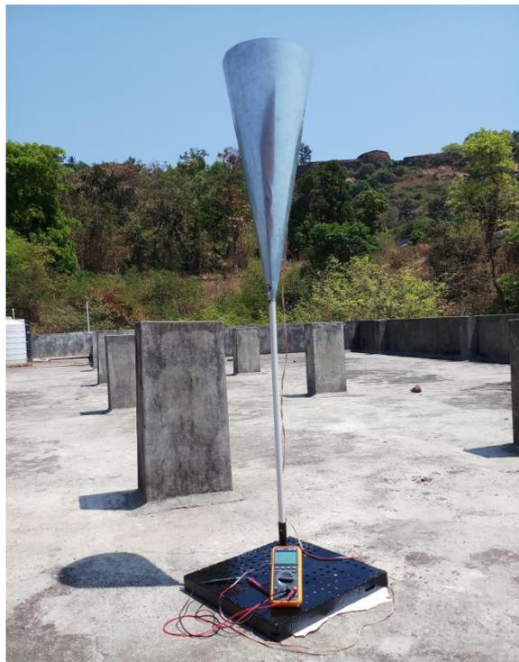
**Fig. Final model of Bladeless Wind Turbine**
