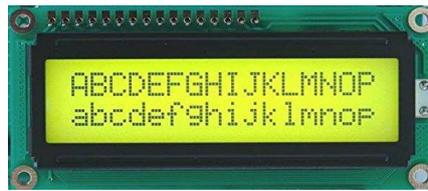
A liquid crystal display (LCD) is a flat, thin display device which is made up of number of monochrome or color pixels which are arrayed in front of reflector or a light source. The features of LCD are Energy efficient, cost effective, Space economy, reduction of radiation and lighter weight.
