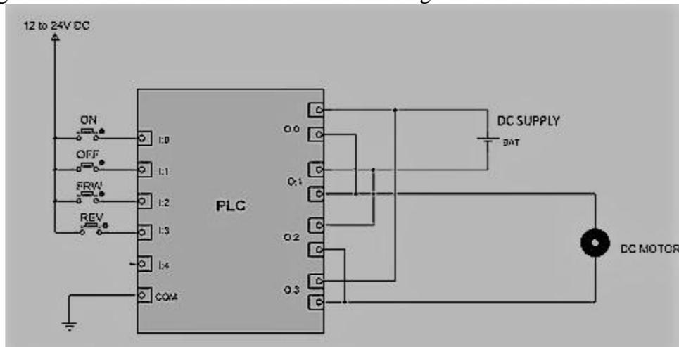
Here is a PLC program to drive motor in forward and reverse direction, along with program explanation and run time test cases.
