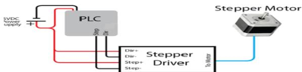
A step motor (or stepper motor as they are commonly referred) is a digital device, in that digital information is processed to accomplish an end result, in this case, controlled motion. It is reasonable to assume that a step motor will faithfully follow digital instructions just as a computer is expected to. This is the distinguishing feature of a step motor.
