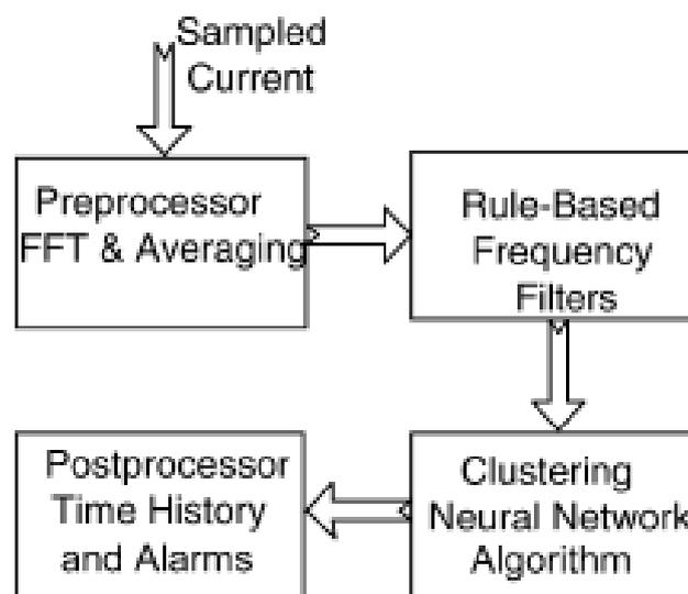
**Fig.1. Block Diagram of ANN based fault diagnosis**
