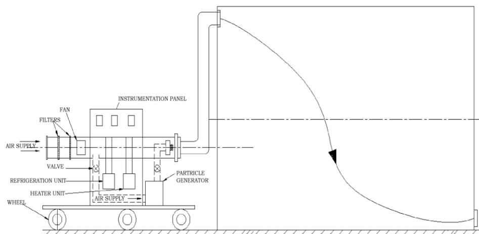
**Figure 3.1** Schematic Diagram of Mixing Ventilated Experimental Test Room and HVAC System
