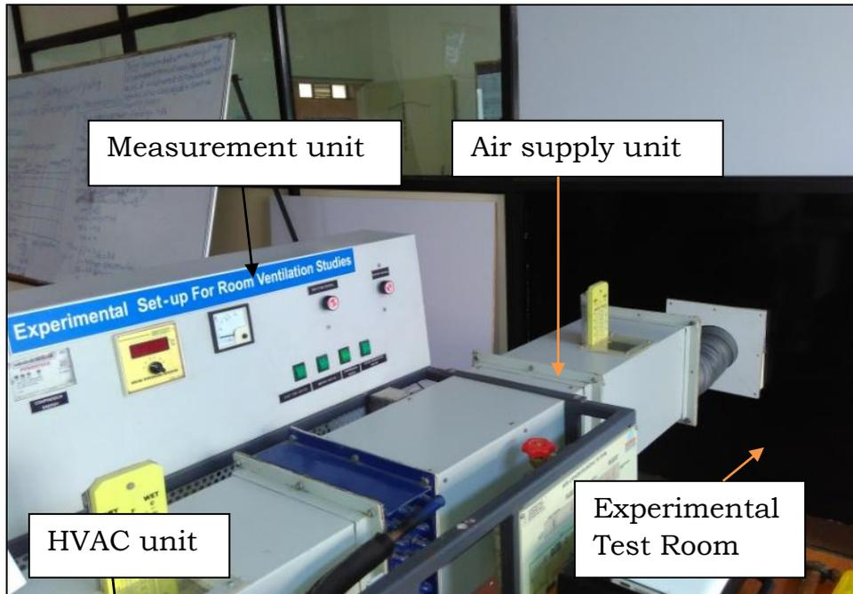
**Figure 3.2** Experimental Set-up for Room Ventilation Studies
