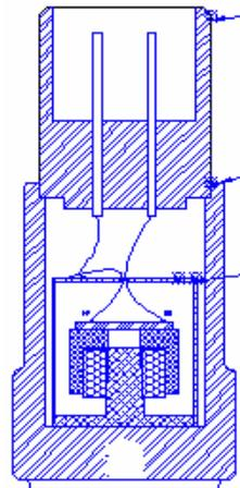
**Fig 2: Triax Accelerometer**
