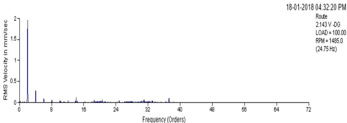
**Fig 17: Vibration of motor at drive end along axial**
