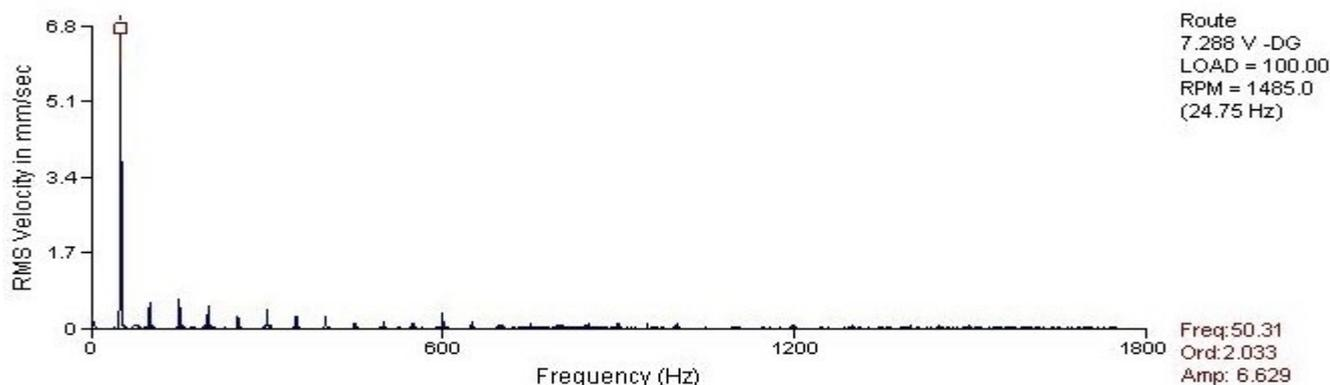
**Fig 4: Vibration of motor at drive end along axial direction.**
