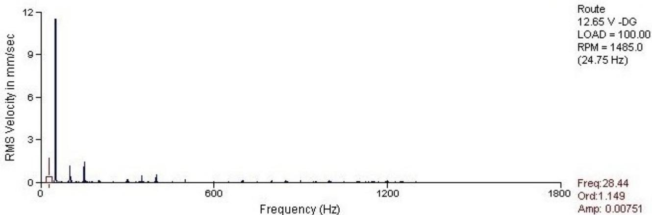
**Fig 3: Vibration of motor at non-drive end along horizontal direction**
