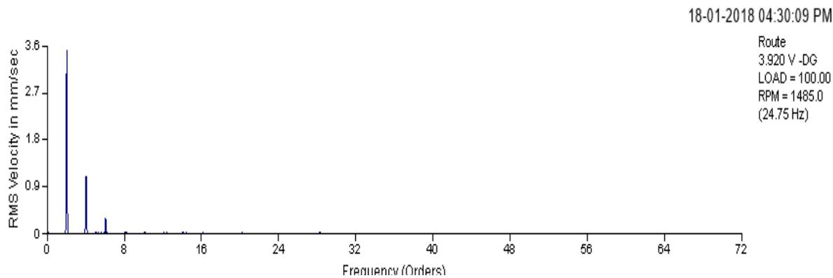
**Fig 16: Vibration of motor at non-drive end along horizontal direction.**
