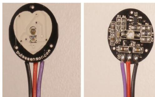
**Fig 1. PULSE SENSOR**
