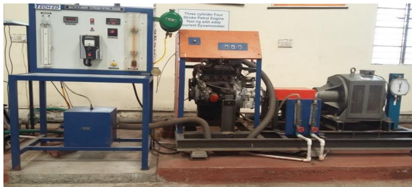
Fig.5: Three cylinder, four stroke, Petrol Engine test Rig with TEG System
