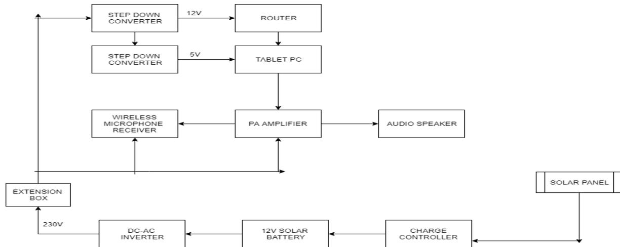
**Figure 4: Block Diagram of the Podium Design**
