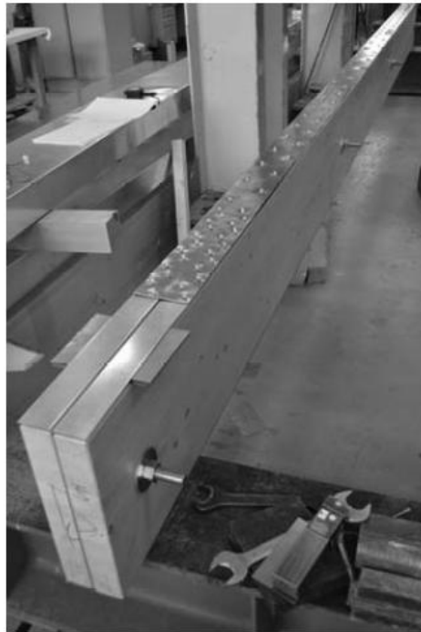
Fig 5: Hybrid timber- Steel beam
