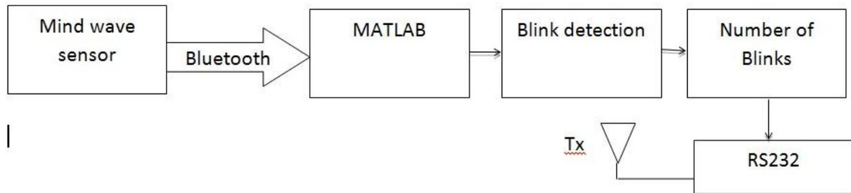
Fig.1: Block Diagram of Proposed System
