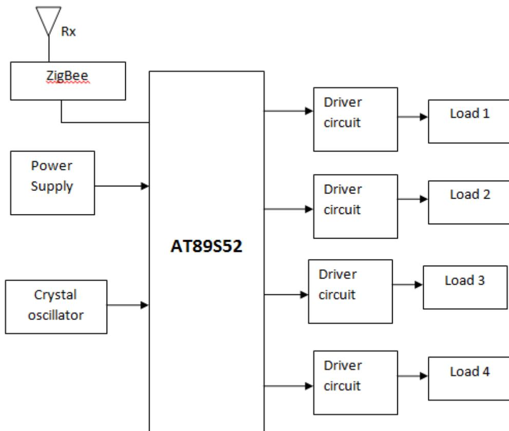
Fig.2: Block Diagram of Embedded System
