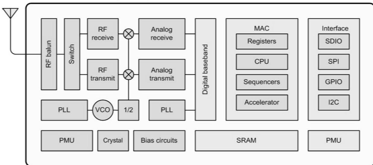
Fig.3: Block Diagram of IOT Module
