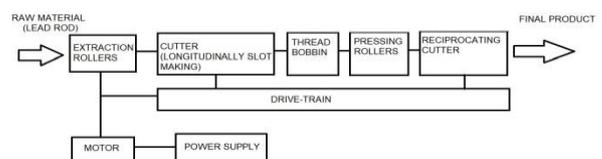
Figure 1: Block diagram of the process
