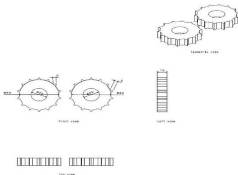
Figure 5.4 : Rotary cutters
