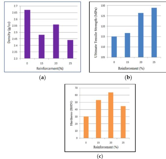
Figure 3. (a) Variation of density with reinforcement (b) Variation of tensile strength with reinforcement (c) Variation of hardness with 4.4.
