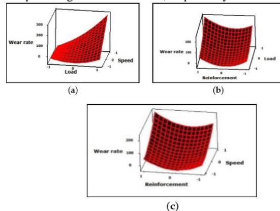
Figure 4. (a) Variation of wear rate with speed and load; (b) Variation of wear rate with load and reinforcement; (c) Variation of wear rate with speed and reinforcement.
