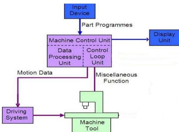
Fig.2. Open loop system
