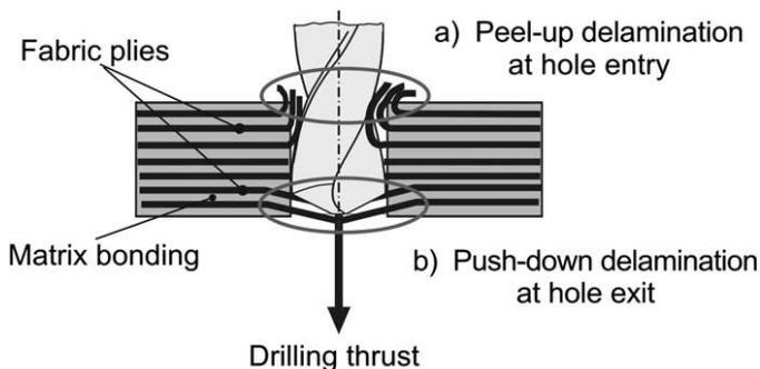
Fig.2. Classification of delamination.
