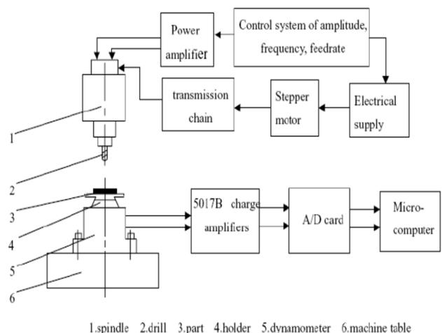
Fig. 4. Schematics of vibration-assisted drilling.
