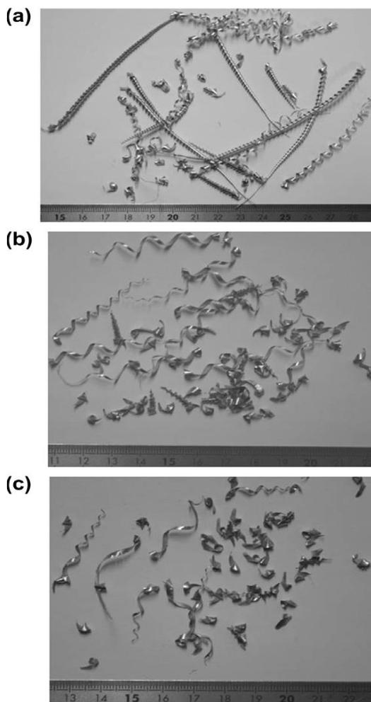
Fig. 3. Influence of the machining parameters on the form of aluminium chips after drilling with coated drill.
