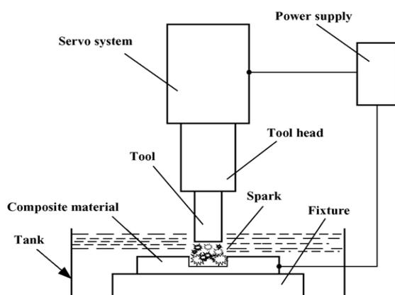
Fig. 5. Schematics of electrical discharge machining.
