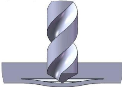
Fig. 1. Delamination mechanism
