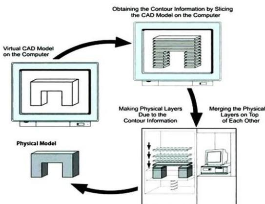
Fig. 2. Printing procedure
