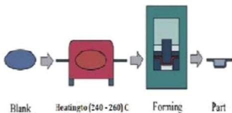
Figure 5.4: Illustration of warm stamping in cold dies process. [4]
