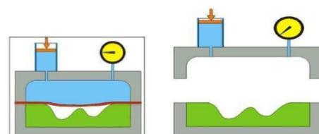
Figure 5.1: Sheet Hydroforming Process. [1]
