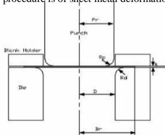
Figure 5.2 Geometrical and Material Parameters. [3]
