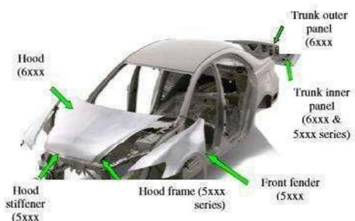
Figure 5.3 Application of aluminium alloy in automotive components
