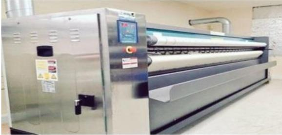
Figure 2. Rolling Press ironing machine
