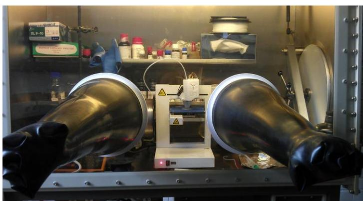
been analyzed in detail. The print of the test specimen according to EN ISO 527-2 (type 1B) as long and thin objects orthogonal to the printing platform revealed certain difficulties. Smaller test specimen (type 1BB, 30 9 2 9 2 mm) would result in a very small printed layer area (4 mm<sup>2</sup>). Consequently, test specimens were printed as small
