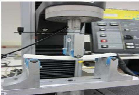
Two metal plates on either side to protect the specimen from the wing nuts and help distribute the load evenly. The specimen was then placed under tensile strength until failure.
