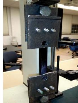
Fig. 2. Flat Orientation print at 80% infill undergoing tensile testing.
