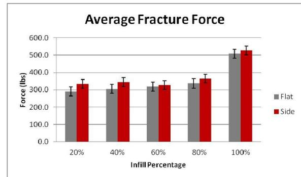
Fig. 1. Average fracture force of both orientations. There is a linear trend from 20%-80% then a rapid increase from 80%-100%. Consistently the side orientation had a higher fracture force than the flat orientation with the strongest fracture force 530.9 lbs.
