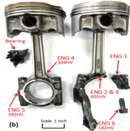
Fig 4. Connecting rod from the motorcycle
