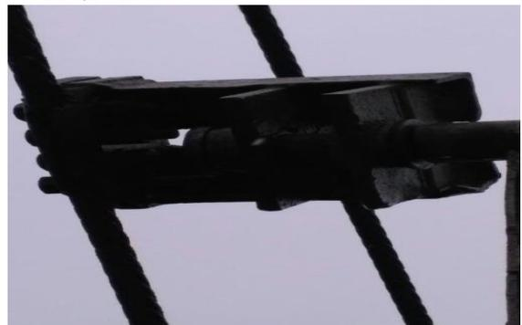
Fig: Gripper attached to the Rope
