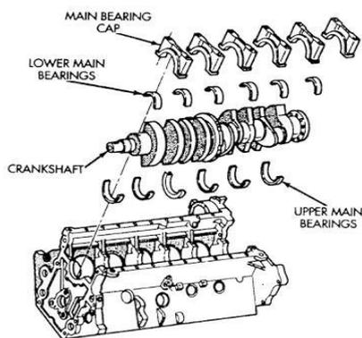
Fig.1 Assembly of Engine Bearing II.
