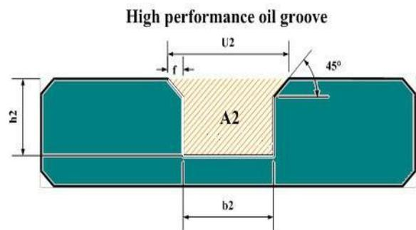
Fig.6 High Performance Oil Groove
