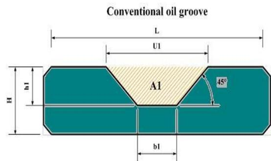
Fig.5 Conventional Oil Groove
