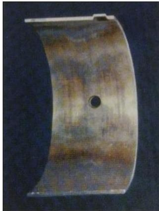
Fig.2 Worn Overlay Surface
