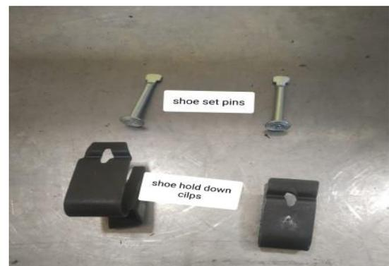
Figure 1 Shoe set pins and clips
