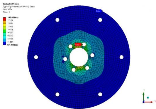
**Figure 4** Thickness = 22 mm, Loading = 250 Kg
