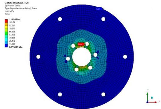
**Figure 10** Thickness = 28 mm, Loading = 250 Kg
