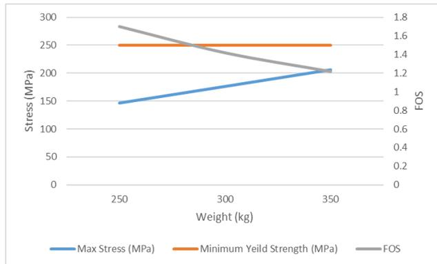
**Figure 14** Analysis of flange with thickness = 25 mm
