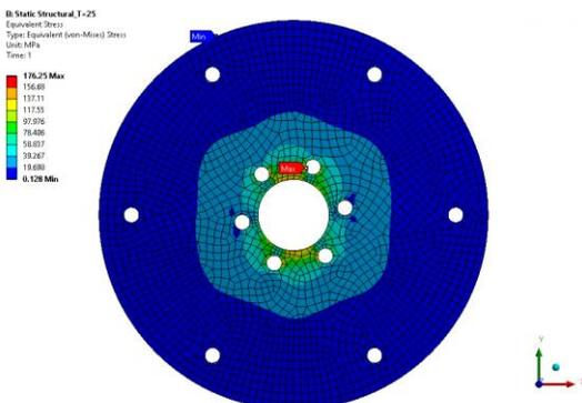
**Figure 8** Thickness = 25 mm, Loading = 300 Kg
