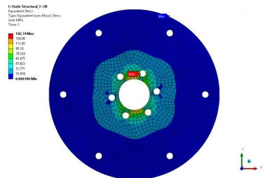
**Figure 11** Thickness = 28 mm, Loading = 300 Kg
