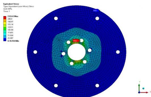
**Figure 5** Thickness = 22 mm, Loading = 300 Kg
