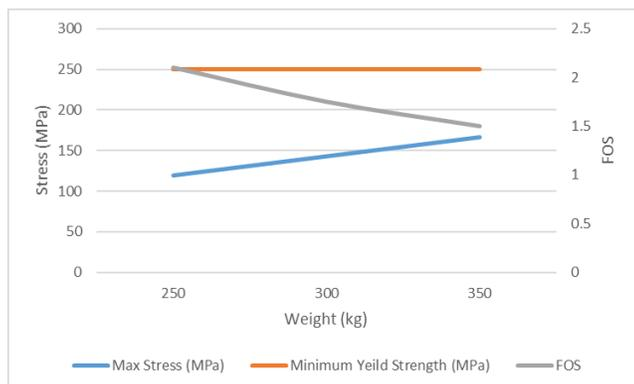
**Figure 15** Analysis of flange with thickness = 28 mm
