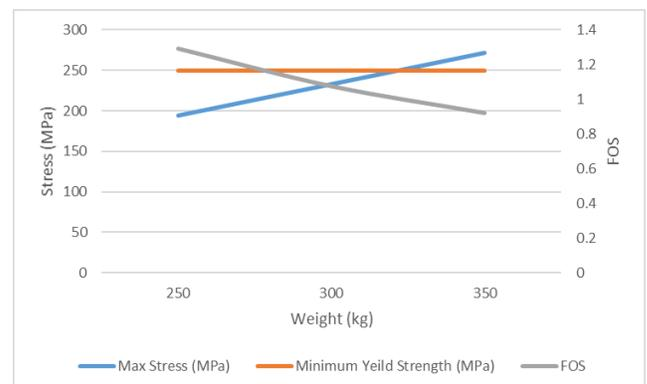
**Figure 13** Analysis of flange with thickness = 22 mm
