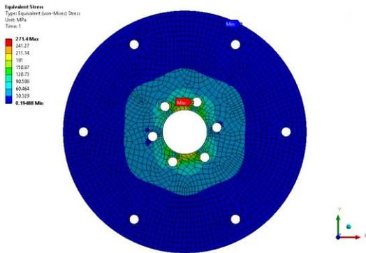
**Figure 6** Thickness = 22 mm, Loading = 350 Kg
