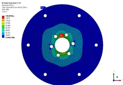
**Figure 7** Thickness = 25 mm, Loading = 250 Kg
