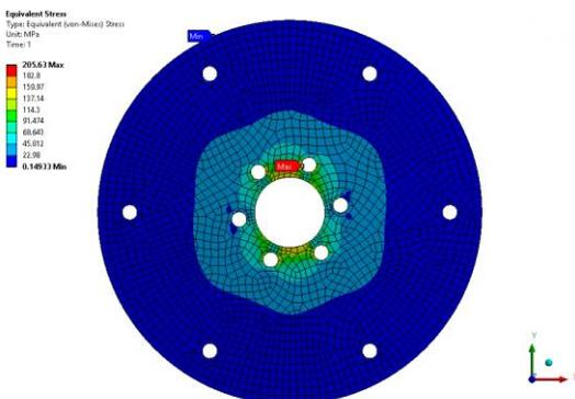
**Figure 9** Thickness = 25 mm, Loading = 350 Kg
