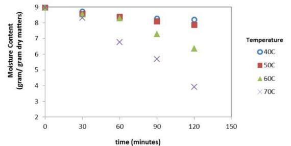
**Fig 4.** Moisture content removal under various drying time and temperatures.
