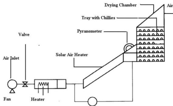
**Fig. 2** Forced convection solar dryer with electric air heater. The above setup consisting of solar dryer and a electric air heater helped determine the important effect on hot air drying and freeze drying kinetics[Fig2].
