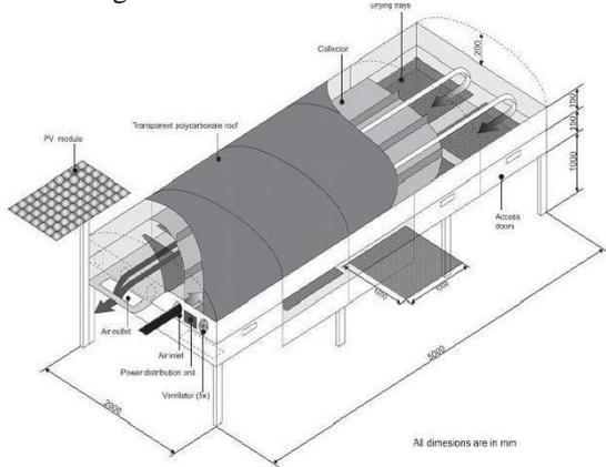
**Fig. 5.** Description of double pass solar dryer.
