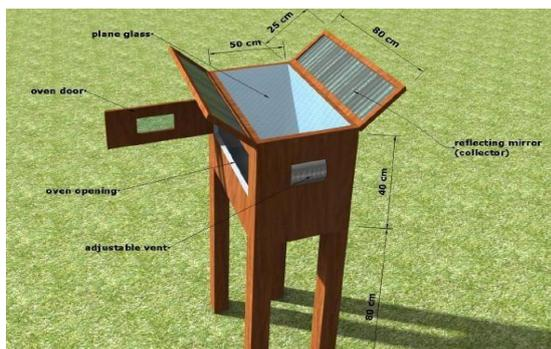
**Fig. 3.** The solar cabinet dryer with mirror reflector
