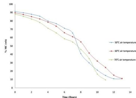
**Fig 1.** Drying curves for mechanical dried red onion slices.
