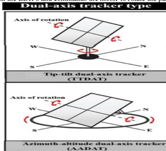
Fig.2 Dual Axis Solar Tracking System
