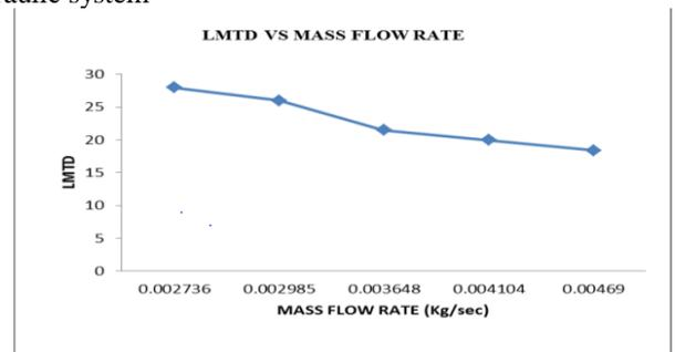
Figure 4:- Effect of logarithmic mean temperature difference (LMTD) of hydraulic system with surrounding v/s mass flow rate fluid in heat pipe.
