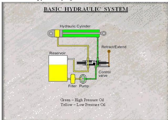
Figure 1 Basic Hydraulic System
