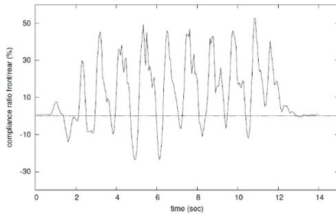
Fig. 3. The average rear leg compliance in respect to the front legs during the stair run.
