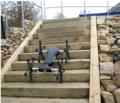
Fig 4. The stair climbing robot
