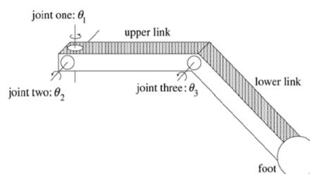
Fig 1 Three-joint leg model.
