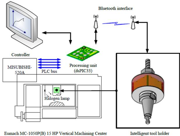
Fig.1 A wireless communication module, a FFT processing unit, internal sensing device, and is capable of monitoring working state of machine tool holder in real time[3].
