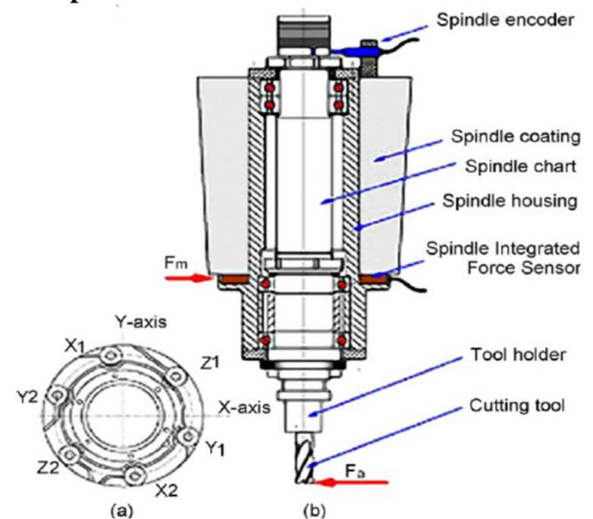
Fig.4 Integrated force sensors in monitor spindle[7]
