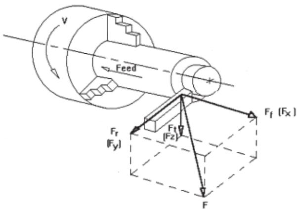
Fig.3 Cutting force components on a single point tool[10].
