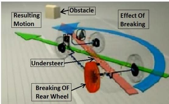
**Fig (a) Working of ESP during avoiding the obstacle.**
