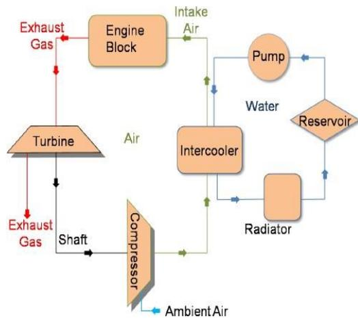
Figure : Turbocharging
